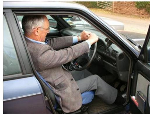
The arm length is adjusted by changing the **squab angle** (3). You should be able to have full and easy access to the whole steering wheel so we need to do checks for that as per the illustration, ensuring the shoulders, and therefore the upper
