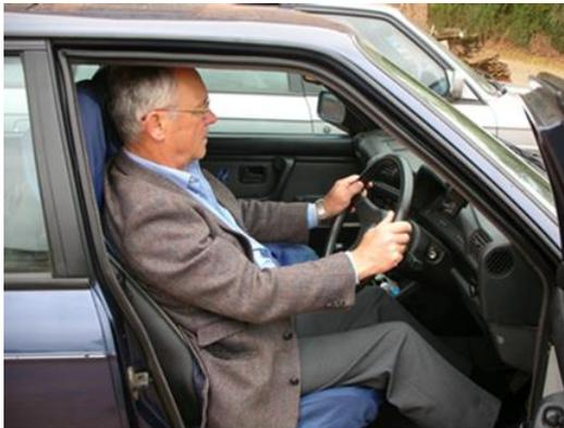
The final adjustment, where possible, is on the steering wheel. Ideally, an extension of its centre-line should meet your body mid-way between the shoulder joints so that there is equal distance from the shoulders to the top or bottom of the wheel.
